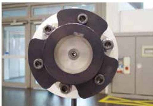
The particular feature on this LP coupling is the bore in the middle. Where long spindles are involved, cooling lubricant can be conducted through this internal tube directly into the work piece.
